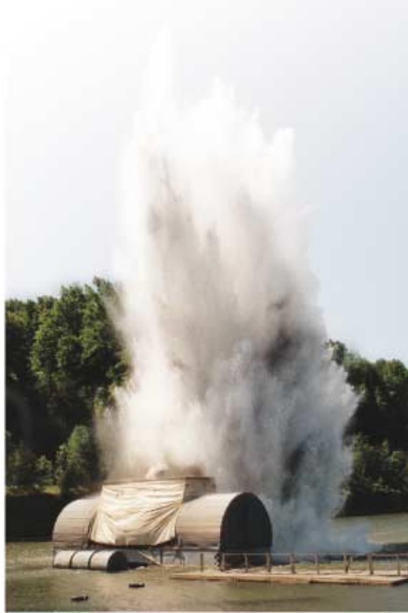
High-shock tests ensure the generator can withstand the force of an enemy attack.
